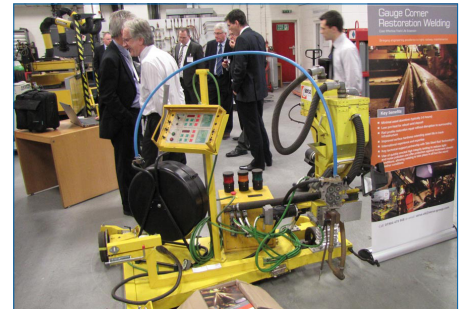
Gauge corner restoration welding equipment
